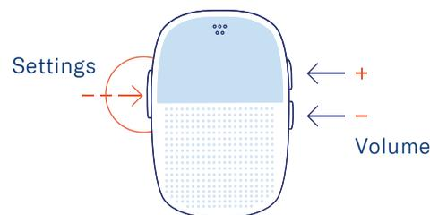
**6. Connecting your phone to the Whisper Brain.** Press the Settings and Volume Up buttons at the same time until the light on the Brain starts pulsing blue. Go to your phone's settings, and connect to the Whisper Brain as you would any other Bluetooth device. For specific instructions on how to do this on your phone model, please visit [whisper.ai/devices](https://whisper.ai/devices).
