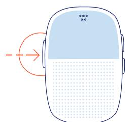
**2. Turning the Whisper Brain on and off.** The Whisper Brain can be turned on or off by pressing and holding the Settings button.
